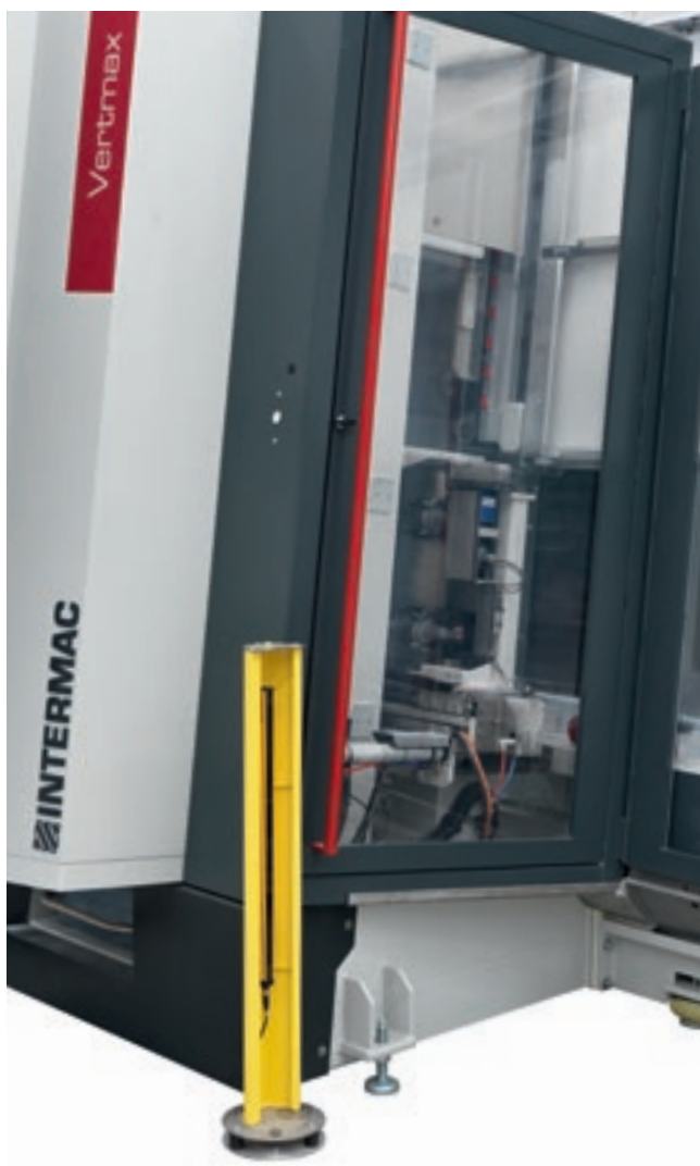
Photocells at the sides of the machine, and anti-intrusion limit switch.
