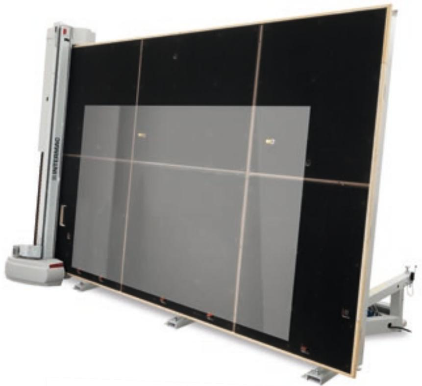
The automatic feet support the sheet while the table is tilting, acting as mechanical sheet aligners when necessary.
