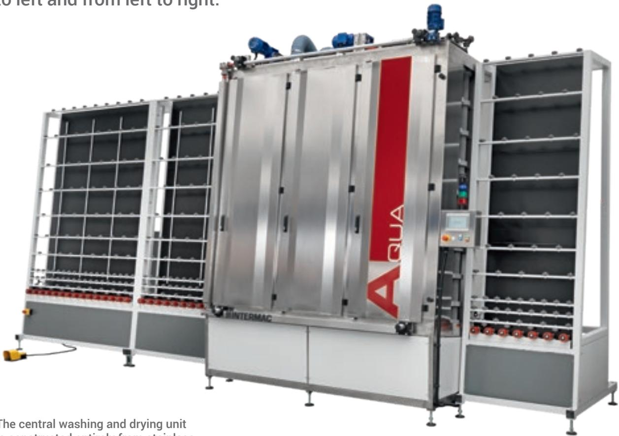
The central washing and drying unit is constructed entirely from stainless steel, guaranteeing safety and durability over time.
