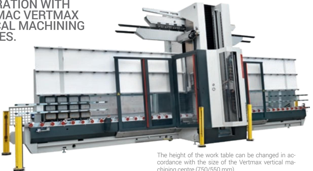
The height of the work table can be changed in accordance with the size of the Vertmax vertical machining centre (750/550 mm).
