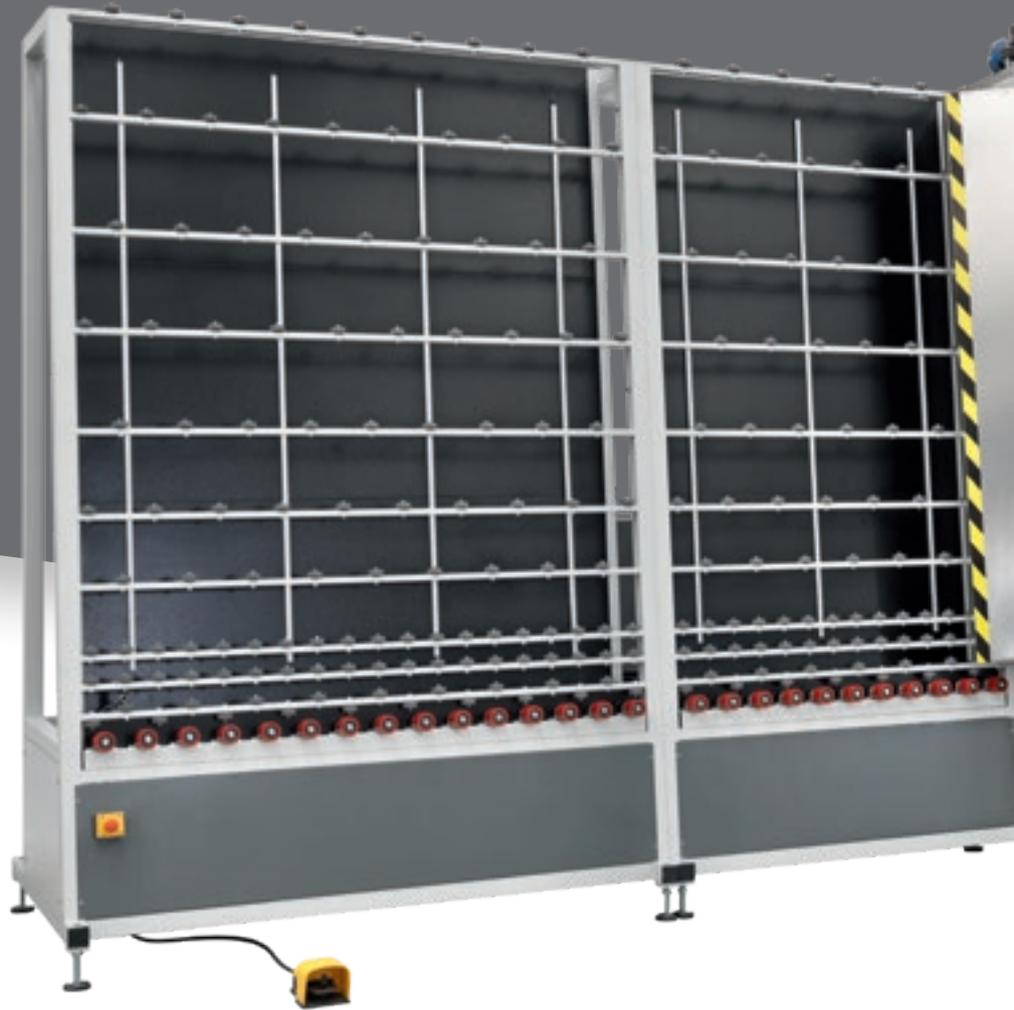
The **Aqua series** is the Intermac range of washing machines which can be fully integrated with vertical machining centres, enabling processed glass to be washed and dried in accordance with the highest standards. Aqua guarantees extreme cleaning of all the impurities accumulated during the machine operations carried out on glass sheets, preparing these perfectly for subsequent processing operations or for leaving the machining cycle.
