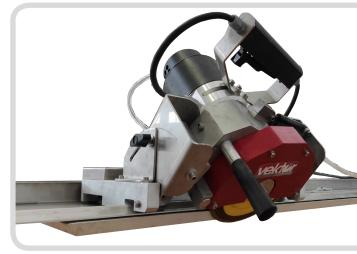
The power of the motor guarantees inclined cuts at 45° up to 3 cm thick on all materials.
