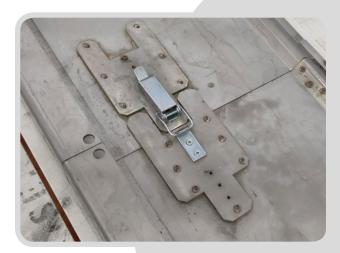
The stainless steel sliding guides can be easily and precisely interconnected and guarantee cuts of any length.
