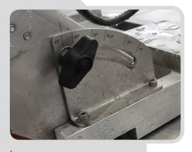
The disc can be inclined up to 45°
