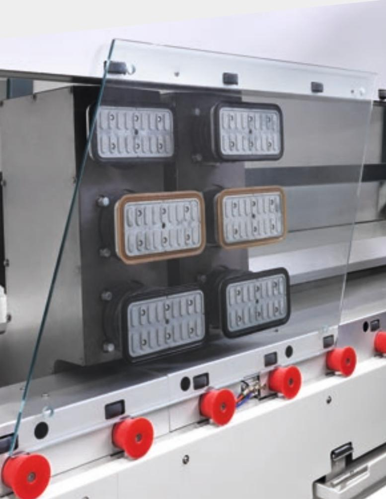
The patented dynamic repositioning system for the suction cup carriages is designed to process a piece without ever leaving it halfway between one suction cup carriage position and the next.
