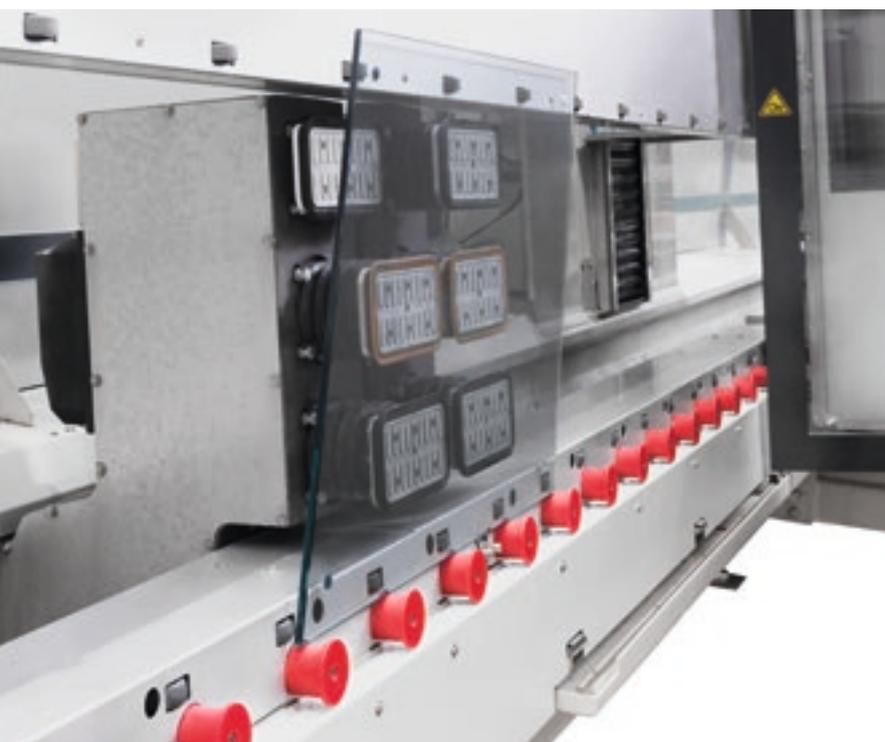
The motorised roller system allows the glass to be loaded at any point, so that the machine can begin to work completely automatically.
