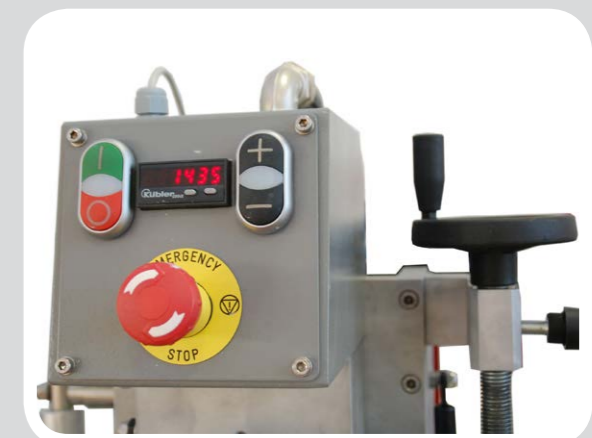
▲ Control panel (24 V AC low tension controls)
