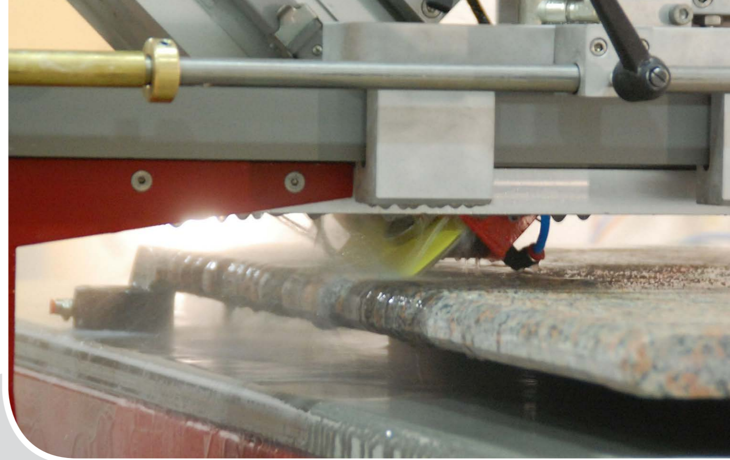
Inclined cuts at 45°
